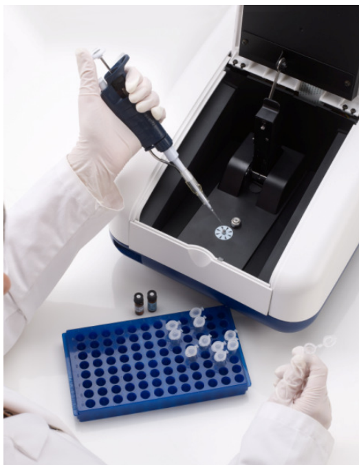
Fig. 1: Applying samples to the read head of the micro volume accessory.
